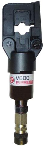
Tested and certified crimp head for crimping Cu-terminals, type KR/KS 10 mm<sup>2</sup>, KRF/KSF 16-150 mm<sup>2</sup>, KRD/KSD 16-185 mm<sup>2</sup>, KRT/KST 10-240 mm<sup>2</sup>, Al-terminals 16-25 mm<sup>2</sup> (-35 solid), C-sleeves 6/6-50/50 mm<sup>2</sup>, DIN 46235 10-95 mm<sup>2</sup>.
