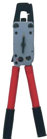
Mechanical hand-held tool for crimping Cu-terminals, type KR/KS 10 mm<sup>2</sup>, KRF/KSF 16-95 mm<sup>2</sup>, KR/D/KSD 16-120 mm<sup>2</sup>, KRT/KST 10-120 mm<sup>2</sup>, Al-terminals 16-25 mm<sup>2</sup> (-35 solid), and C-sleeves 6/6-50/50 mm<sup>2</sup>, DIN 46235 10-95 mm<sup>2</sup>.
