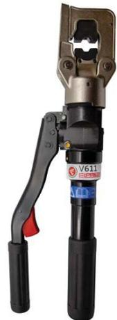
Tested and certified hand-held tool for crimping Cu-terminals, type KR/KS 10 mm<sup>2</sup>, KRF/KSF 16-150 mm<sup>2</sup>, KRD/KSD 16-185 mm<sup>2</sup>, KRT/KST 10-240 mm<sup>2</sup>, Al-terminals 16-25 mm<sup>2</sup> (-35 solid), C-sleeves 6/6-50/50 mm<sup>2</sup>, DIN 46235 10-95 mm<sup>2</sup>.
