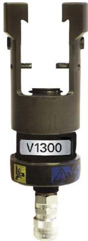
Tested and certified crimp head for crimping Cu-terminals, type KR/KRT 10 mm<sup>2</sup>, KS/KST 10 mm<sup>2</sup>, KRF/KRD/KRT 16-400 mm<sup>2</sup>, KSF/KSD/KST 16-400 mm<sup>2</sup>, Al-terminals 16-400 mm<sup>2</sup> (-240 solid), DIN 46235 10-300 mm<sup>2</sup>, C sleeves up to 240 mm<sup>2</sup> total area (C95-120). Used in combination with foot pump P4000 or the electrically powered pump PS710 (battery powered version of PS710E is also available).
