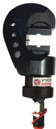
Tested and certified crimp head for crimping Cu-terminals, type KR/KRT 10 mm<sup>2</sup>, KS/KST 10 mm<sup>2</sup>, KRF/KRD/KRT 16-400 mm<sup>2</sup>, KSF/KSD/KST 16-400 mm<sup>2</sup>. Used in combination with foot pump P4000 or battery and mains powered pump PS710 (battery powered version of PS710E is also available).
