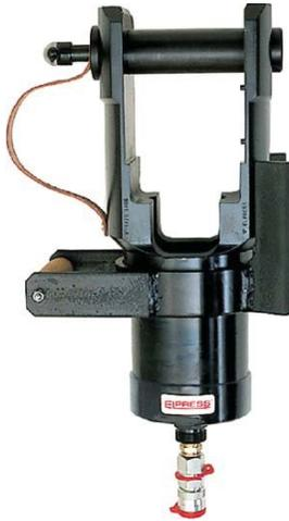
Tested and certified crimp head for contact crimping Cu-terminals, type KRF/KSF 500-800 mm<sup>2</sup>, KRK/KSD, KRT/KST 500-1000 mm<sup>2</sup>, Al-terminals 800-1200 mm<sup>2</sup>, C-sleeves 245-540 mm<sup>2</sup> (C150-185 och C240-300). Used in combination with foot pump P4000 or electrically powered pump PS710.
