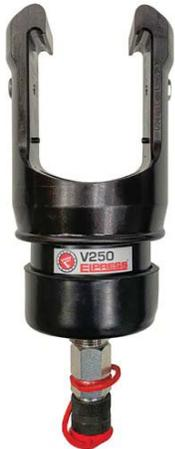
Tested and certified crimp head for crimping Cu-terminals, type KR/KRT 10 mm<sup>2</sup>, KS/KST 10 mm<sup>2</sup>, KRF/KRD/KRT 16-800 mm<sup>2</sup>, KSF/KSD/KST 16-800 mm<sup>2</sup>, Al-terminals 16-630 mm<sup>2</sup> (-300 solid), C sleeves 6/6-300/300 mm<sup>2</sup>. Used in combination with foot pump P4000 or the electrically powered pump PS710 (battery powered version of PS710E is also available).
