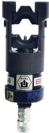
Tested and certified crimp head with patented DUAL technology for crimping Cu-terminals, type KR/KRF and KS/KSF 10-300 mm<sup>2</sup>. Used in combination with foot pump P4000 or the electrically powered pump PS710 (battery powered version of PS710E is also available).
