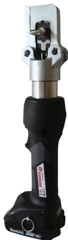
Tested and certified battery-powered crimp tool for crimping Cu-terminals, type KR/KS 10 mm<sup>2</sup>, KRF/KSF 16-150 mm<sup>2</sup>, KR/D/KSD 16-185 mm<sup>2</sup>, KRT/KST 10-240 mm<sup>2</sup>, Al-terminals 16-25 mm<sup>2</sup> (-35 solid), C sleeves 6/6-50/50 mm<sup>2</sup>, DIN 46235 10-95 mm<sup>2</sup>. PVX611DB has an extra battery.
