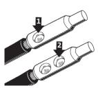
Matrix holder TV2620, matrix TP13M, punch TP13D. Crimp sequence
